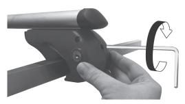
**PLEASE NOTE:** When installing the roof bars, please ensure the mounting bracket is securely connected to the roof rails, as shown below (A). If roof bars are incorrectly mounted (as shown in B & C, this will risk destabilising the load, causing danger to other road users).
