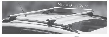
**5.** Once both roof bars have been mounted and correctly positioned, secure them with the security keys to cover the Allan key access with the red guard.
